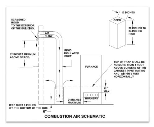
There are two methods for sizing outdoor combustion air. The first method requires an opening to the outside within 12 inches of the ceiling of the furnace room, with a size of 1 square inch for every 3000 BTUs of input.
