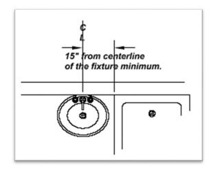
A minimum of 24 inches shall be provided in front of a toilet, bidet, or lavatory to any wall, partition, door, or any other fixtures.
