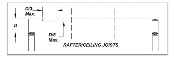
Notches on the ends of sawn lumber shall not be notched over one-fourth the depth of the member.
