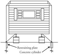
A vertical anchor can be made more resistant to horizontal displacement by installing a steel plate next to it or by casting a concrete cylinder around the upper portion of the rod.
