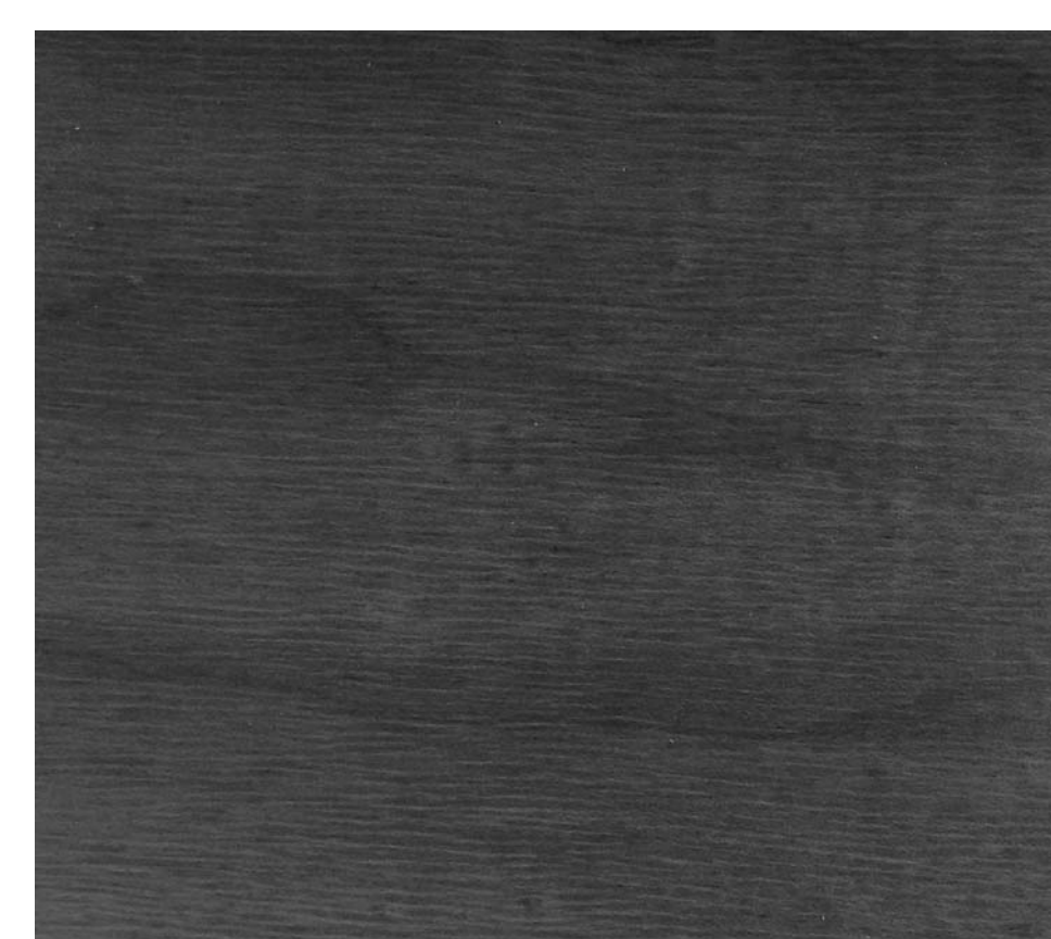
MEDIUM STAINED MAPLE AS BASIS OF DESIGN FOR ALL WOODS UNLESS NOTED OTHERWISE. NOTE: WOOD STAINS TO MATCH EXISTING STAINS BEING USED THROUGHOUT THE PROJECT.
